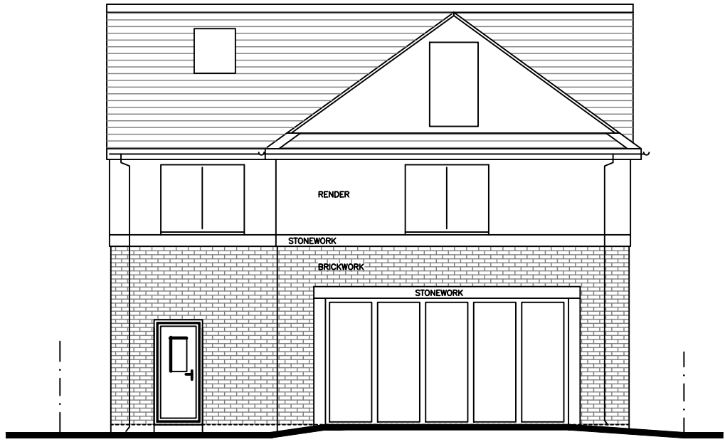
EXISTING REAR ELEVATION
